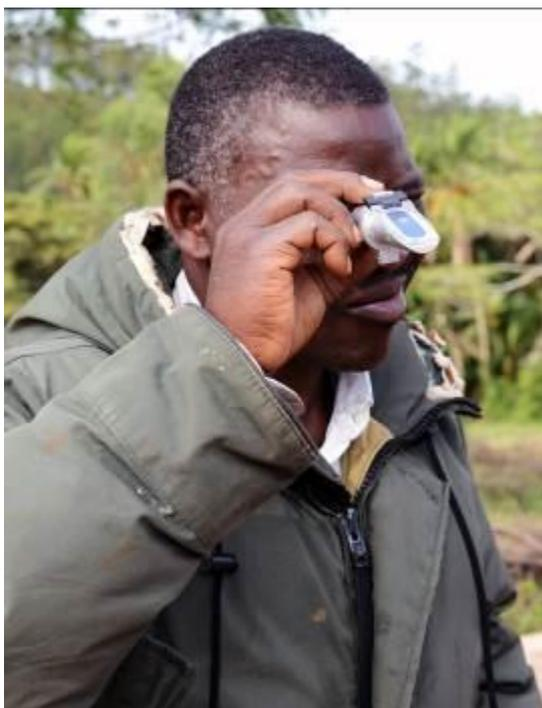
FIGURE 19: USING A BRIX METER
