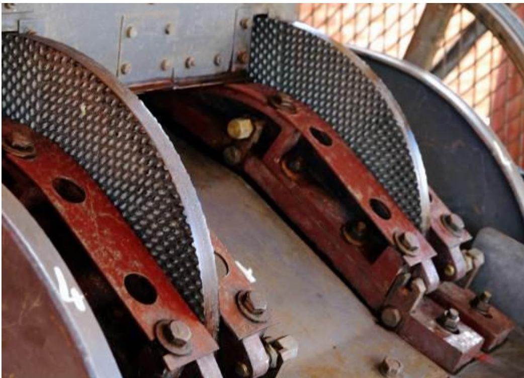
**FIGURE 27: CLEAN AND WELL MAINTAINED DISC PULPER AT WASHING STATION**
