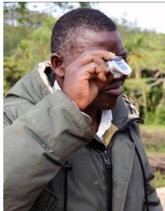
**FIGURE 19: USING A BRIX METER**
